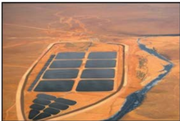
Figure 9. Aerial view of the Mzab wastewater stabilization system. Photo Credit: Bouchama, 2022, https://doi.org/10.1007/978-3-031-03600-2_2
