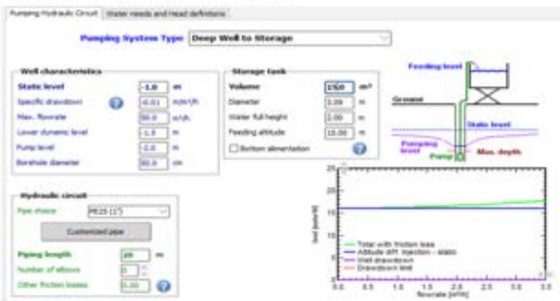
Figure 7 : Pumping Hydraulic Circuit from PVsyst
