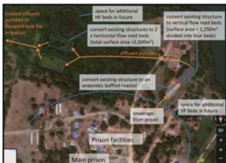
Figure 19. An aerial map of the current layout incorporating the CW and the location of the HF-CW beds. Photo Credit: UNEP & Nairobi Convention, 2019, https://nairobi.convention.org/clearinghouse/node/395
