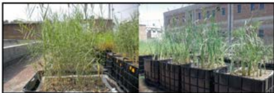
Figure 25. Floating CWs with bacterial inoculants to decompose dye-rich wastewater. Photos Credit: Mustafa & Afzal, 2022, https://doi.org/10.1007/978-3-031-03600-2_13
