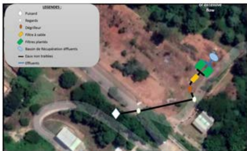
Figure 5: Overview of the treatment system
