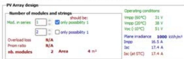
Figure 12 : PV system configuration from PVsyst
