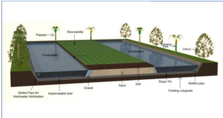
Figure: Proposed freshwater rice permaculture lagoon with Surface Flow design Source: Finarch – 2024 (Author)
